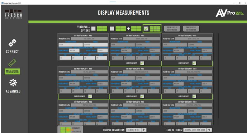
**NOTE:** If all displays are the same make and model, next check the “COPY DISPLAY 1” boxes. The display info from the DISPLAY-1 box will be auto entered into the other display rectangles.
