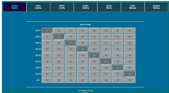
Across the top of the page you will see different tabs for Sense Switching (HDMI Matrix), Video Setting, HDCP Config, Audio Setting, Audio Matrix, EDID Manage, and System Settings. Simply choose the tab that corresponds with what you would like to configure. The rest is a matter of you choosing what you would like the switch to do. All of the different functions (plus a few more) of the Matrix Switch we've described so far in this Quick Start Guide can be done easily in the web interface.
