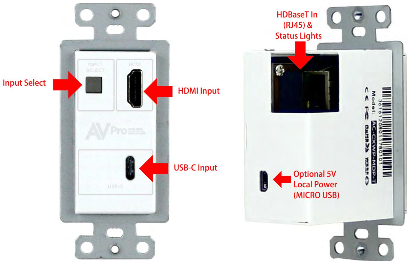
There is one Indicator light on the front of the AC-CXWP-USBC-T (INPUT SELECT) and 2 on the HDBaseT Port
